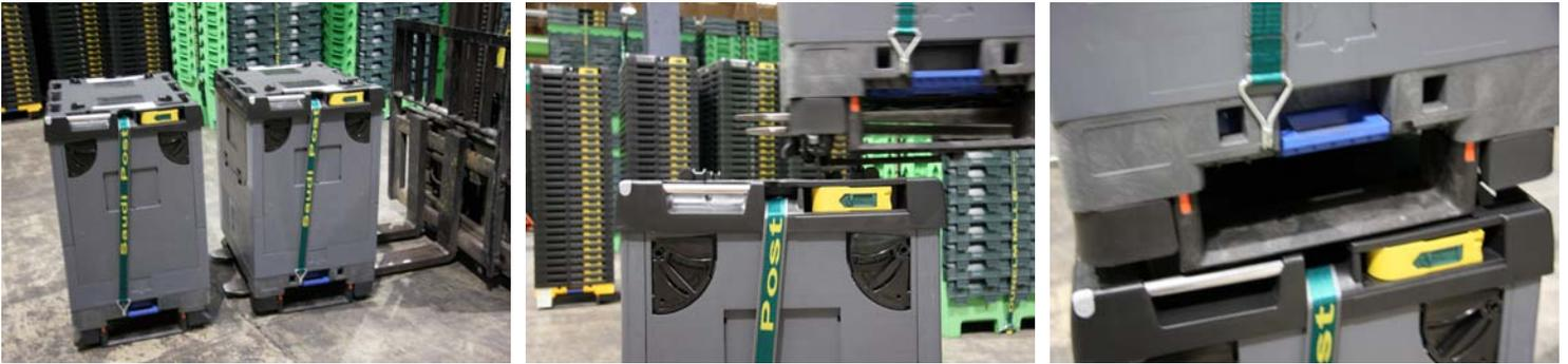
Make sure that you strap the 2 units using the straps from the top lid. This is very important to insure perfect stability. The 2 units are now safe to be moved either with a fork lift or manually.
